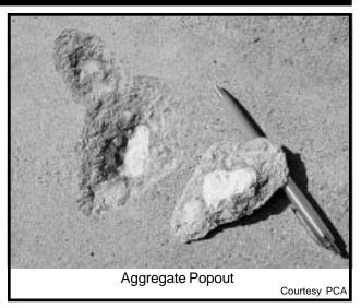
tural concrete in severe exposure, allow several types of particles which may cause popouts when exposed to freezing and thawing in the saturated condition. The most common type of particles resulting in popouts are low density chert in natural aggregate deposits.
